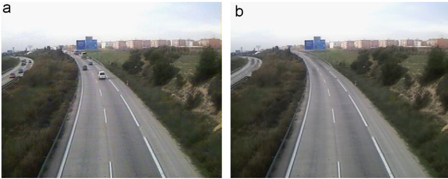
Fig. 1. (a) One image of a sequence and (b) its estimated background.
