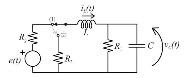
Data: e(t)=10V,  $R_g=R_1=1\Omega$ ,  $R_2=2\Omega$ , L=1H, C=2F.
