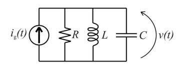
$\frac{d}{dt} \left\{ i_R(t) + i_L(t) + i_C(t) = i_g(t) \right\}$ (Charge conservation)  $\Rightarrow \frac{1}{R} \frac{dv(t)}{dt} + \frac{1}{L}v(t) + C \frac{d^2v(t)}{dt^2} = \frac{di_g(t)}{dt}$  $\Rightarrow \frac{d^2v(t)}{dt^2} + \frac{1}{RC} \frac{dv(t)}{dt} + \frac{1}{LC}v(t) = \frac{1}{C} \frac{di_g(t)}{dt}$
