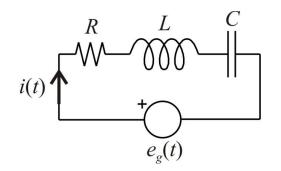
$\frac{d^2 i(t)}{dt^2} + \frac{R}{L}\frac{di(t)}{dt} + \frac{1}{LC}i(t) = \frac{1}{L}\frac{de_g(t)}{dt}$  $\Rightarrow \omega_n = \frac{1}{\sqrt{LC}}, \xi = \frac{R}{2\omega L}$
