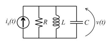
$$\frac{d^2 v(t)}{dt^2} + \frac{1}{RC} \frac{dv(t)}{dt} + \frac{1}{LC} v(t) = \frac{1}{C} \frac{di_g(t)}{dt}$$
