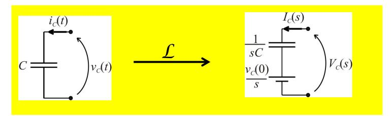
$$\begin{split} I_{C}(s) &= \mathcal{L}[i_{C}(t)], \\ V_{C}(s) &= \mathcal{L}[v_{C}(t)], \\ V_{C}(s) &= \int_{0}^{\infty} v_{C}(t)e^{-st}dt = \frac{1}{C}\int_{0}^{\infty} q(t)e^{-st}dt = \frac{1}{C}\left(\frac{q(0)}{s} + \frac{1}{s}I_{C}(s)\right) \\ &= \frac{1}{sC}I_{C}(s) + \frac{v_{C}(0)}{s}. \end{split}$$
