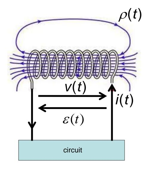
The time varying flux  $\rho(t)$  produces a voltage as shown in the figure
