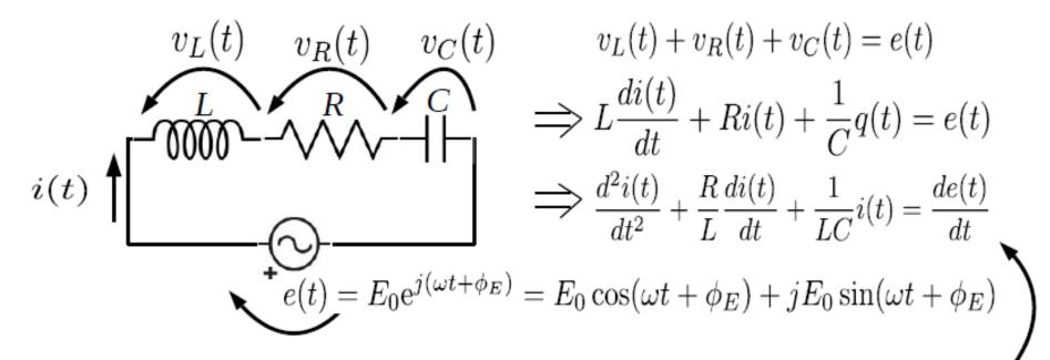
To solve the circuit means to solve the 2<sup>nd</sup> order differential equation 16
