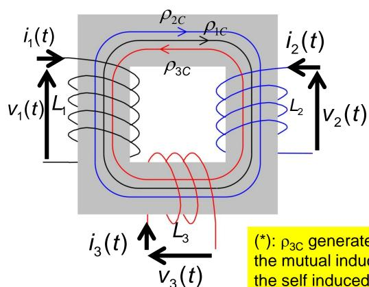
$$\begin{cases} v_{1} = L_{1} \frac{d}{dt} i_{1} + M_{12} \frac{d}{dt} i_{2} - M_{13} \frac{d}{dt} i_{3} \\ v_{2} = L_{2} \frac{d}{dt} i_{2} + M_{21} \frac{d}{dt} i_{1} - M_{23} \frac{d}{dt} i_{3} \\ v_{3} = L_{3} \frac{d}{dt} i_{3} - M_{31} \frac{d}{dt} i_{1} - M_{32} \frac{d}{dt} i_{2} \\ M_{12} = K_{12} \sqrt{L_{1}L_{2}}, \\ M_{23} = K_{23} \sqrt{L_{2}L_{3}}, \\ M_{13} = K_{13} \sqrt{L_{1}L_{3}}. \end{cases}$$
