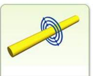
When an electric current runs through a wire, an electromagnetic field is generated around it.
