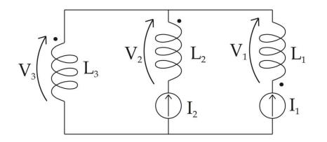
$$\begin{cases} V_{1} = -j\omega L_{1}I_{1} + j\omega M_{12}I_{2} - j\omega M_{13}(I_{1} + I_{2}) \\ V_{2} = -j\omega L_{2}I_{2} + j\omega M_{12}I_{1} + j\omega M_{23}(I_{1} + I_{2}) \\ V_{3} = j\omega L_{3}(I_{1} + I_{2}) + j\omega M_{13}I_{1} - j\omega \omega_{23}I_{2} \end{cases}$$
