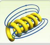
gh By winding the wire into a tighter coil, the field is made stronger, i.e., higher current and more number of wire turns produce a stronger field.
