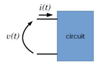
$$\implies P = \frac{1}{T} \int_0^T \frac{1}{2} V_0 I_0 \cos(\phi_V - \phi_I) dt + \frac{1}{T} \int_0^T \frac{1}{2} V_0 I_0 \cos(2\omega t + \phi_V + \phi_I) dt = 0$$
