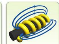
The field can be made stronger by placing an iron bar in the coil center, thus, increasing the power of the electromagnet.
