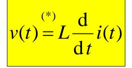
(\*) Note that the voltage is pointing to the terminal whose current is entering the coil
