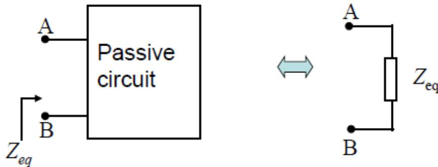
The equivalent impedance can be obtained by:
