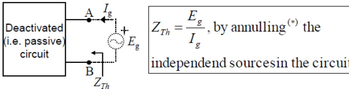
(\*): Voltage source replaced by short circuit
