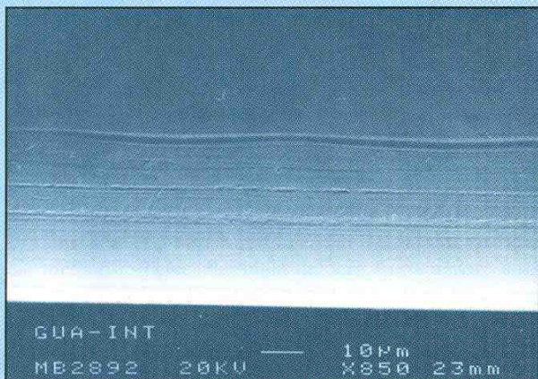
Fig. 5. An SEM view (850x) of the test wire presented in Figs. 3 and 4 reveals a corresponding series of longitudinal defects.
